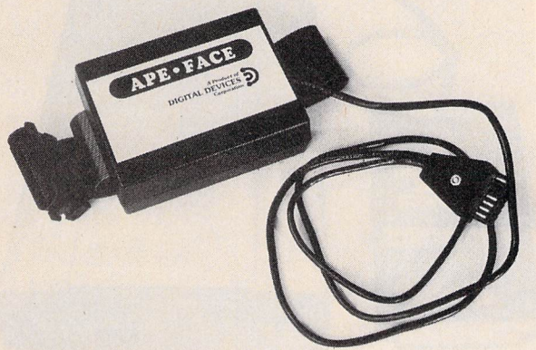
APE FACE from Digital Devices Corp., converts a non-standard Atari printer output to standard Centronics.
